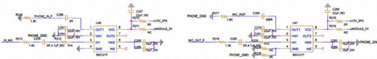
图7 智能照护机器人交互系统的数字音频降噪电路图 Fig.7 Circuit diagram of digital audio denoising for intelligent care robot interaction system
