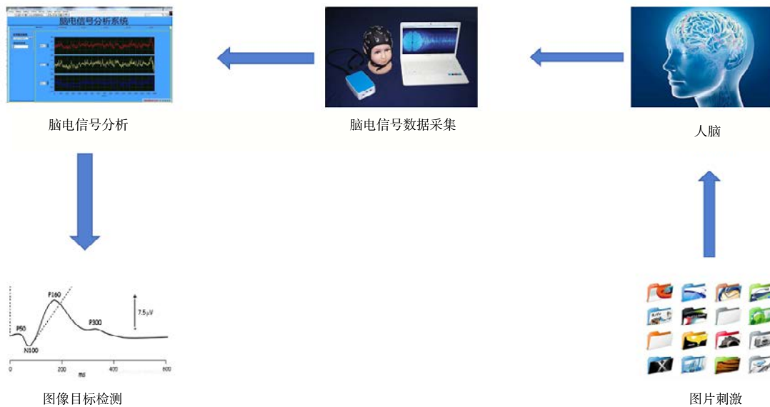
图 3 基于 ERP 信号的目标检测的基本流程 Fig.3 Basic process of target detection based on ERP signal
